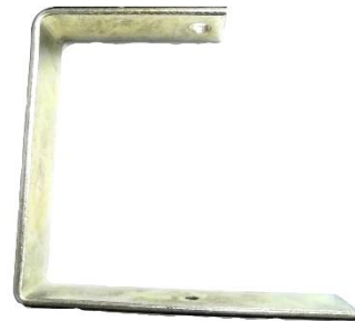
A-MAX 3"x6" Trunking Bracket (Premium) 150mm(L) x 32mm(W) x 125mm(H) 4.5mm(thickness) x 32mm(W) flat bar
