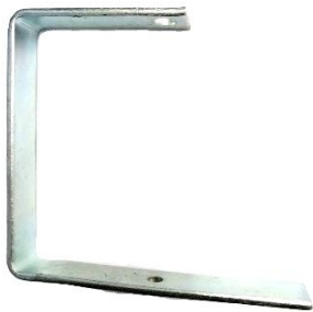
A-MAX 3"x6" Trunking Bracket (Eco) 150mm(L) x 25mm(W) x 125mm(H) 4.5mm(thickness) x 25mm(W) flat bar
