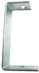
A-MAX 2"x2" Trunking Bracket 50mm(L) x 25mm(W) x 100mm(H) 2.8mm(thickness) x 25mm(W) flat bar
